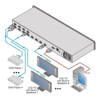
Figure 3: Connecting the VS-48HN 4x8 HDMI Matrix Switcher
