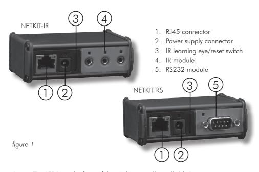
3 mm. The LED's on the front of the Netkit unit will rapidly blink in unison, indicating a reset. Use a light touch when resetting your Netkit unit, as force may damage your Netkit hardware irreparably.
