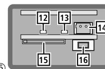
The LED (12) will light up when a card has been inserted.
