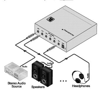
Figure 8: Connecting the VM-50HN Headphone Distributor
