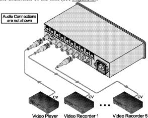
Figure 7: Connecting the VM-5S Video Audio Distributor
