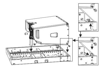
In stacked installation (for example a line-array stacked on a S318 sub), the use of the pins, of the rear bracket of VIO-L210, and of the 2 movable bars of DRK-210, as shown, make the assembling quick and easy.
