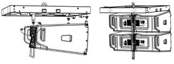
As shown in the picture, in flown installation, the use of the pins and of the rear bracket of DRK-210 make the assembly with the first element of the line-array simple and safe.
