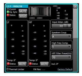
Those VIO L210 parameters can be controlled by using dBTechnologies Network:
