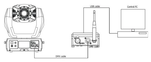
To upload software into the fixture.
