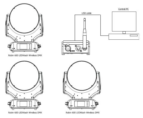
To link moving heads to the Robe Universal Interface WTX, press the wireless link button on the Robe Universal Interface WTX.
