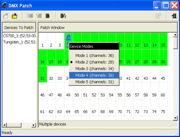
Use the same process for all fixtures in list of fixtures. The properly assigned DMX channels are green, red channels indicate overlapping channels, yellow channels indicate that some channels will be missing.
