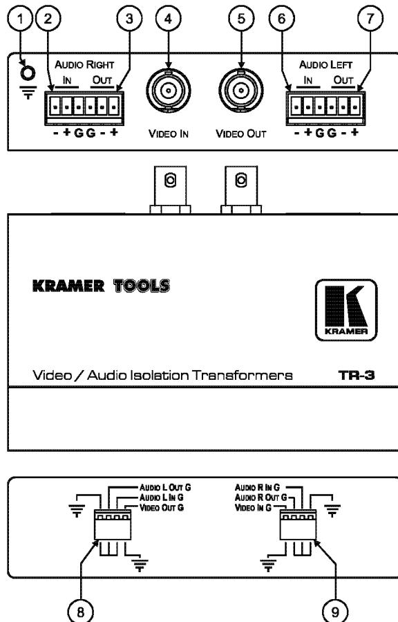
*Figure 4: TR-3 Video / Audio Isolation Transformers*
