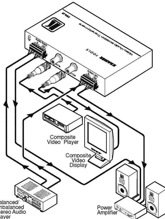
*Figure 5: Connecting the TR-3 Video / Audio Isolation Transformer*
