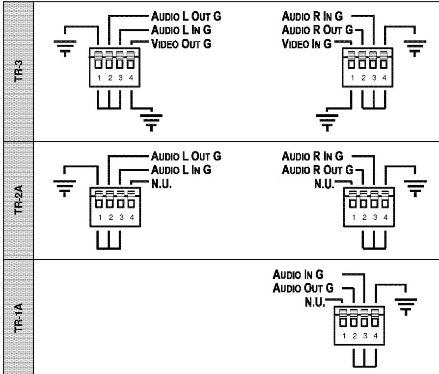
Figure 6: Dipswitch Settings for TR-3, TR-2A and TR-1A
