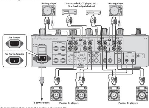
To use the fader start function, connect a control cable (page 12).
