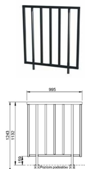
**SBS 06 - steel handrail 1m**
