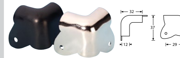
CABINET CORNER WITH CUTAWAY 2 LEG 1 mm Steel, Fixing holes \varnothing 4.2 mm, weight 17 g.
