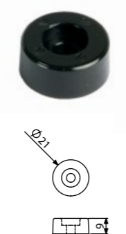
4926 PLASTIC STACKING FOOT MALE black plastic foot, \varnothing 21 mm, Fixing hole \varnothing 5.1 mm PLASTIKSTAPELFUSS MALE Schwarzer Kunststoff, \varnothing 21 mm, Befestigungsloch \varnothing 5,1 mm ► For use with / passend zu: 4925
