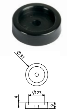
4925 PLASTIC STACKING FOOT FEMALE black plastic foot, \varnothing 32 mm, Fixing hole \varnothing 5.1 mm PLASTIKSTAPELFUSS FEMALE Schwarzer Kunststoff, \varnothing 32 mm, Befestigungsloch \varnothing 5,1 mm ► For use with / passend zu: 4926
